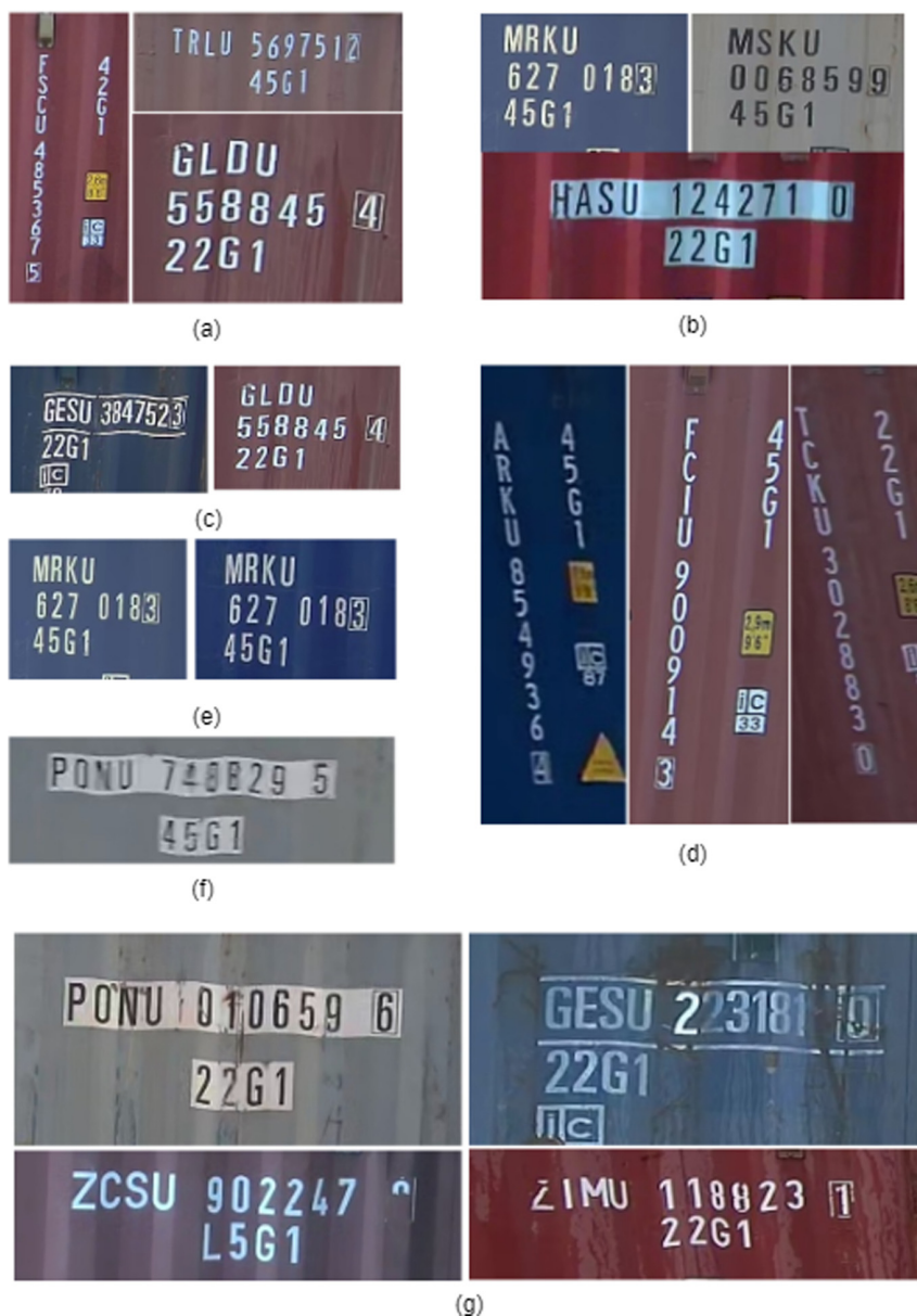
Fig. 2. Hindering factor examples (a) Different formats (horizontal/vertical letters, 2/3 lines) (b) Color of background (dark/bright), color of letters (white/black) and letters in a box (c) Inclined letters due to the rough surface (d) Different camera angles (e) Different brightness (day/night time, artificial lighting) (f) Blurry, noisy images (g) Letters' quality (rusted, deformed, discolored) (Color figure online)
